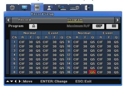
Two choices are available: 1) Select a program by the frame rate, quality, and resolution, or 2) Set up a program manually. For Event Recording, you can select a frame rate up to the maximum possible for one channel. When events occur simultaneously in more than two channels, the recording frame rate may be automatically adjusted.
